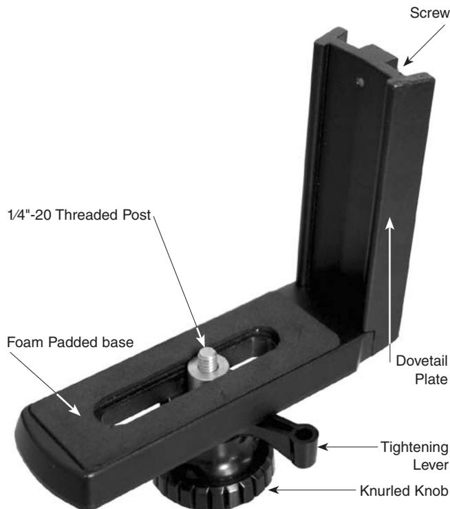
**Figure 4.** The TeleTrack Mount 1/4"-20 L-bracket
