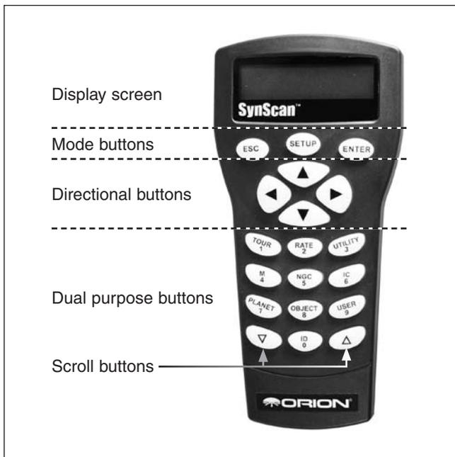
**Figure 6:** The TeleTrack AZ-G hand controller
